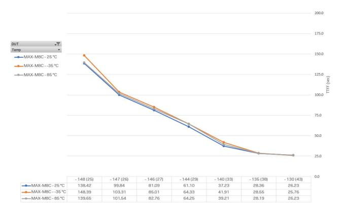
Figure 3: TTFF vs. signal power in dBm and equivalent C/N0 inside parenthesis for MAX-M8C during cold starts at +25, -35, and +85 °C (default mode: GPS & GLONASS including QZSS, SBAS)
