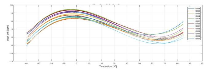
Figure 1: Temperature effect crystal on various crystal-based modules
