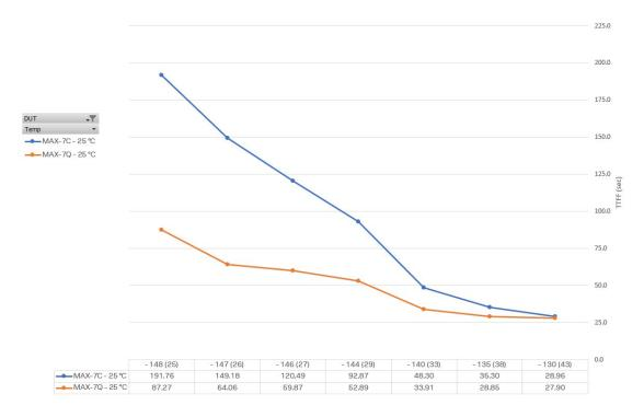
Figure 10: TTFF vs. signal power in dBm and equivalent C/N0 inside parenthesis for MAX-7Q and MAX-7C during cold starts 18
