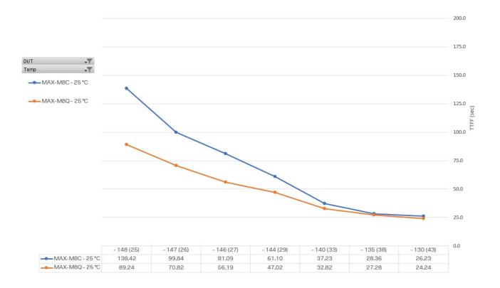
Figure 2: TTFF vs. signal power in dBm and equivalent C/N0 inside parenthesis for MAX-M8Q and MAX-M8C during cold starts<sup>7</sup> (default mode: GPS & GLONASS including QZSS, SBAS)
