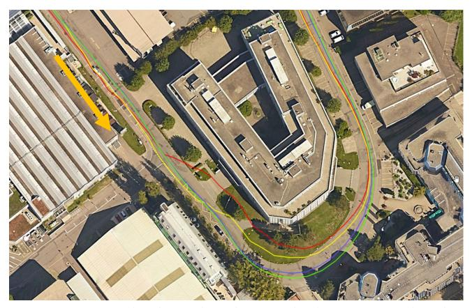
Figure 15: Tracks for MAX-M8C (in blue), MAX-7Q (in yellow), and MAX-7C (in red), and reference position (in green) in a narrow street
