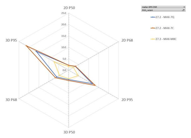
Figure 13: Position error in meters for MAX-M8C, MAX-7Q and MAX-7C in percentiles at 27.2 dBHz in a rural area
