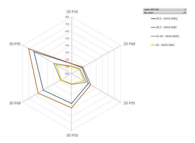
Figure 9: Position error in meters for MAX-M8C and MAX-M8Q in percentiles at 28.5 and 42 dBHz in a highway test (default mode: GPS and GLONASS including QZSS, SBAS)
