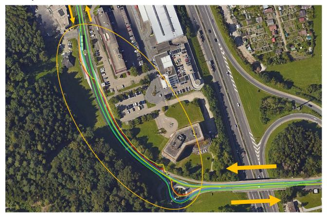
Figure 14: Tracks for MAX-M8C (in blue), MAX-7Q (in yellow), and MAX-7C (in red), and reference position (in green) in an area with lower GNSS visibility
