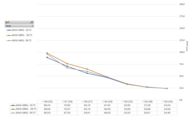
Figure 4: TTFF vs. signal power in dBm and equivalent C/N0 inside parenthesis for MAX-M8Q during cold starts at +25, -35, and +85 °C (default mode: GPS & GLONASS including QZSS, SBAS)
