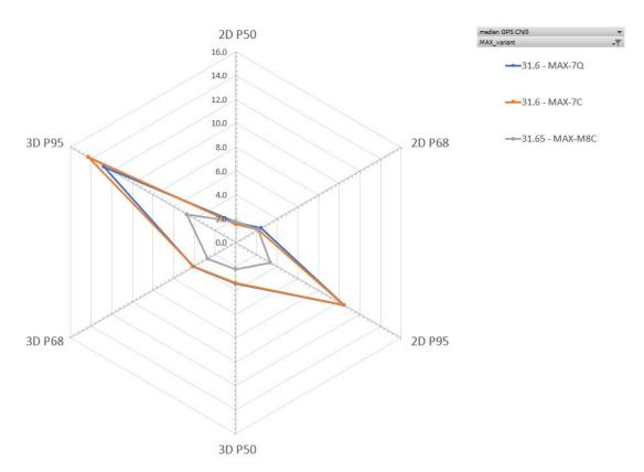
Figure 12: Position error in meters for MAX-M8C, MAX-7Q and MAX-7C in percentiles at 31.6 dBHz in a rural area
