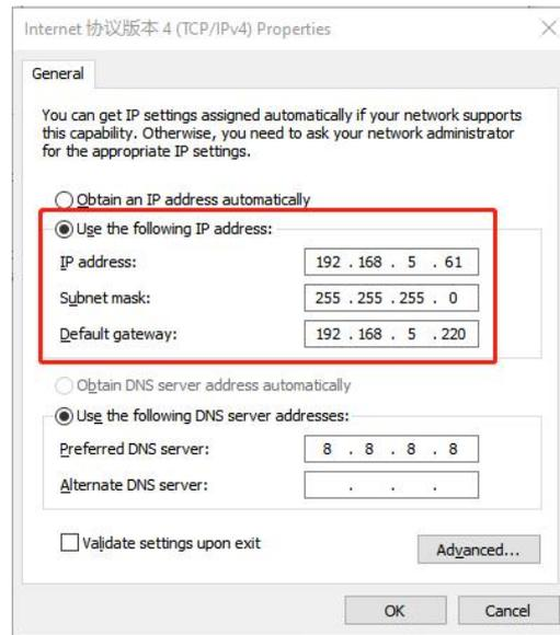
Step 3: Open the Browser and type 192.168.5.220 to access the web GUI. After logging on web GUI successfully, user is allowed to view configuration page.
