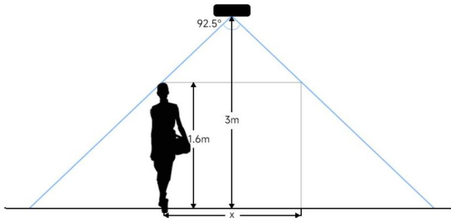
For example, if the Minimum height of pedestrians is 1.6 m, the detection area corresponding to each installation height is as follows:
