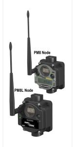
The Sure Cross® wireless system is a radio frequency network with integrated I/O that operates in most environments to eliminate the need for wiring runs.
