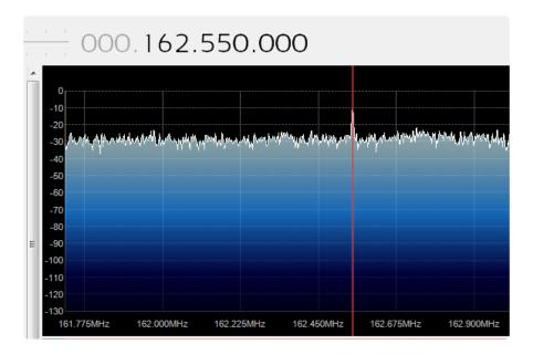
You can see a little peak, its much smaller signal than the FM radio stations. It's also much thinner which makes it a narrow-band FM rather than wideband. Since its voice, not stereo music, they use less of the frequency band, so select **NFM** as the decoding type
