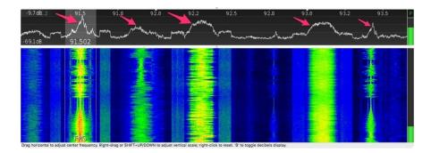
The frequency band for FM broadcast radio is 88MHz to 108MHz.
