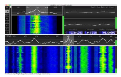
You can see the fine tuning section in the upper left corner gives us a zoomed in view of the demodulator. You can drag this one left and right in the waterfall section to fine tune, or grab one of the outer edges of the demodulator to change the bandwidth that is being processed. Too wide and you'll pick up unwanted signals, too narrow and you'll start to cut off important parts of the signal.
