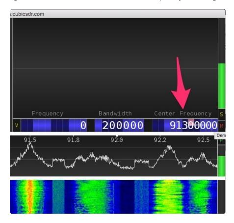
This will bring a range of frequencies into view -- approximately 3MHz at a time are available. Now, you can set a demodulator down on a range you want to tune. This is done by clicking in the waterfall display, with the cursor at the center of the
