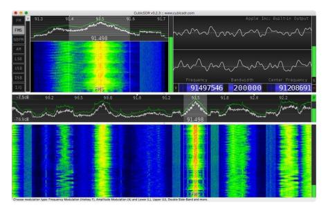
First, make sure your RTL device has started by clicking the **File > Stop / Device** menu item. When it is running you will see the waterfall frequency display moving at the bottom of the interface, as well as some moving waveforms in the other areas.
