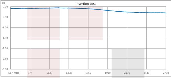
2 Way High Power Equal Tapper with 4.1/9.5 Mini DIN Operating from 600 MHz to 2.7 GHz Rated at 300 Watts from Fairview Microwave is in-stock and available to ship same-day. All of our RF/microwave products are available off-the-shelf from our ISO 9001:2008 certified facilities in Allen, Texas. Fairview Microwave is RF on-demand.
