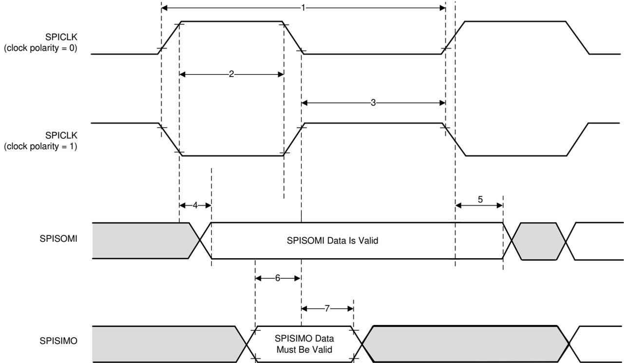
**Figure 6-12. SPI Peripheral Mode External Timing (CLOCK PHASE = 0)**
