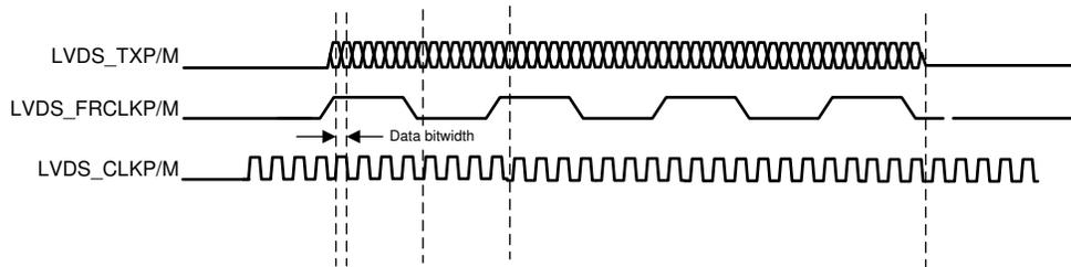
**Figure 6-15. LVDS Interface Lane Configuration And Relative Timings**
