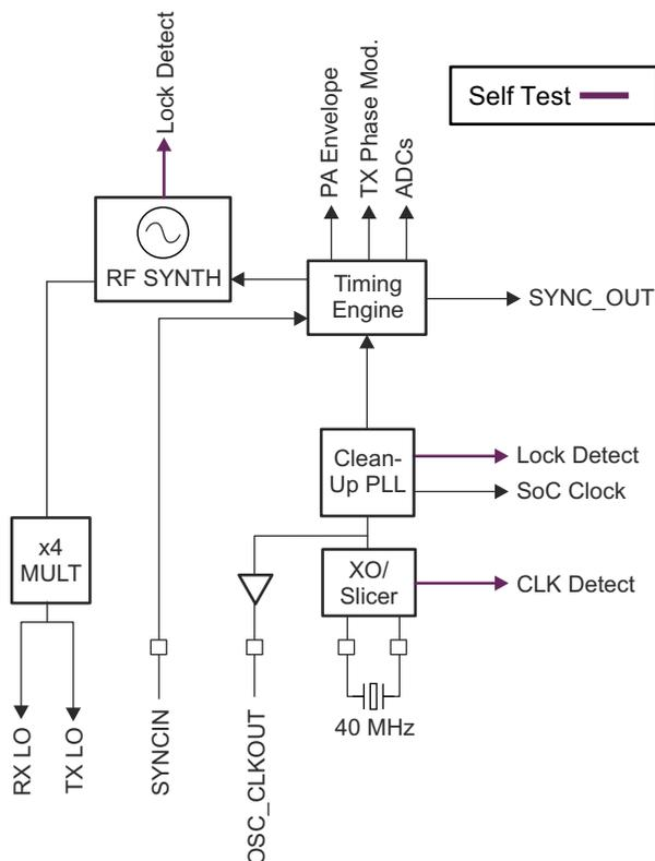
Figure 7-1. Clock Subsystem
