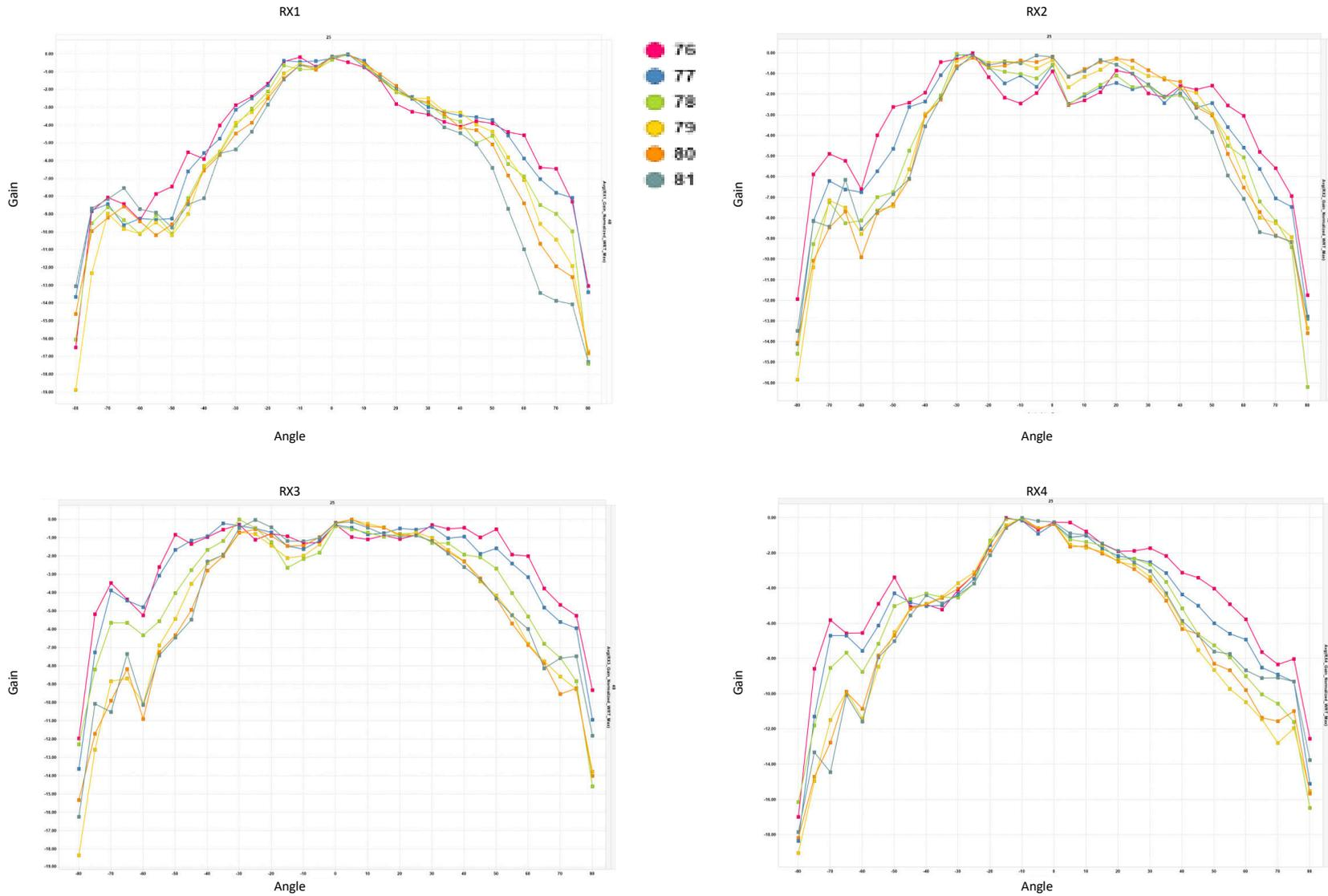
Figure 6-2. Receiver Antenna Radiation Pattern - Azimuth
