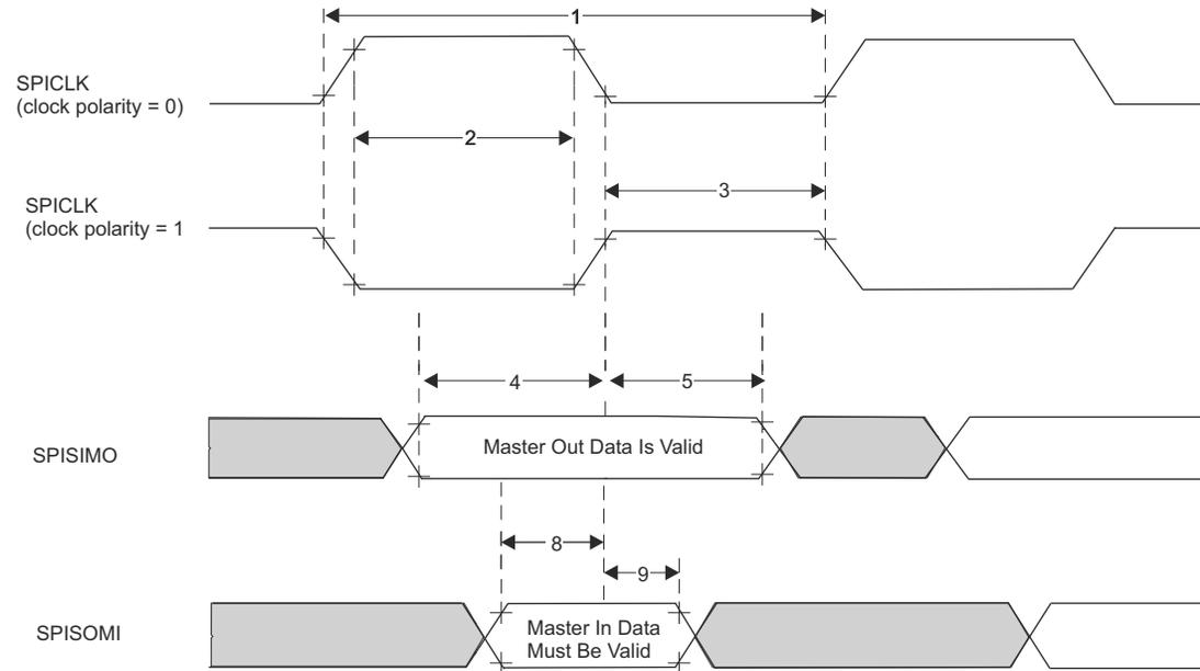
**Figure 6-8. SPI Controller Mode External Timing (CLOCK PHASE = 0)**
