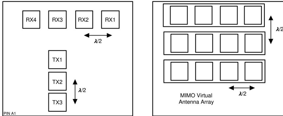
**Figure 6-5. Antenna Positions (Placement and Relative Spacing)**
