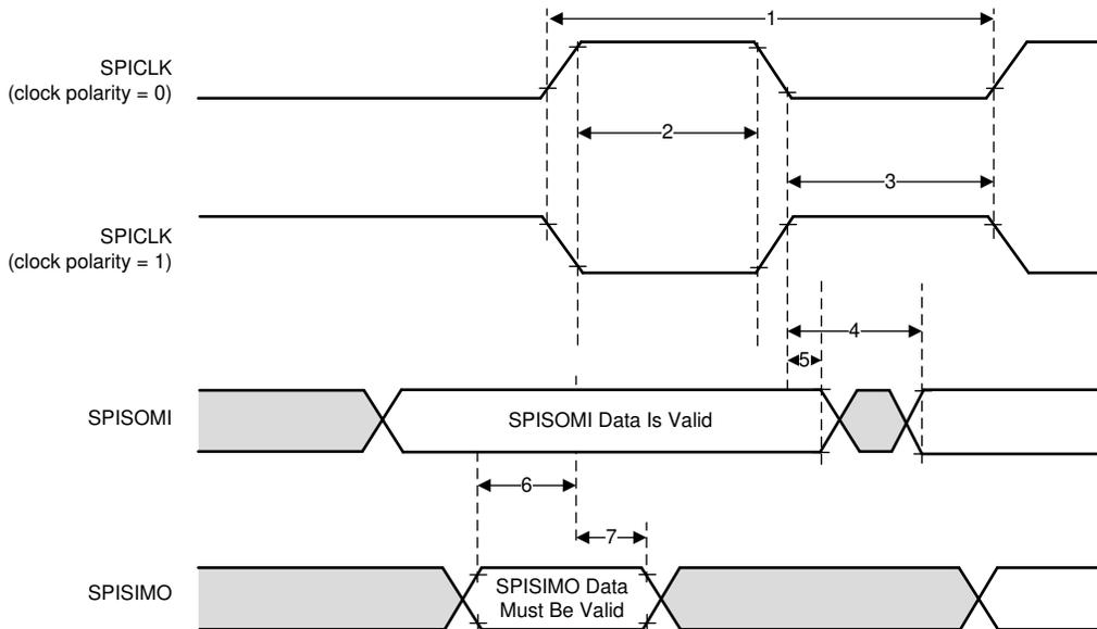
**Figure 6-13. SPI Peripheral Mode External Timing (CLOCK PHASE = 1)**
