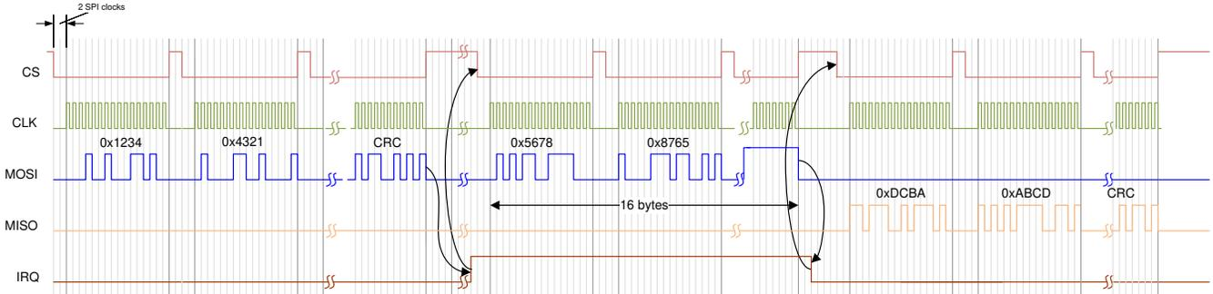
**Figure 6-14. SPI Communication**
