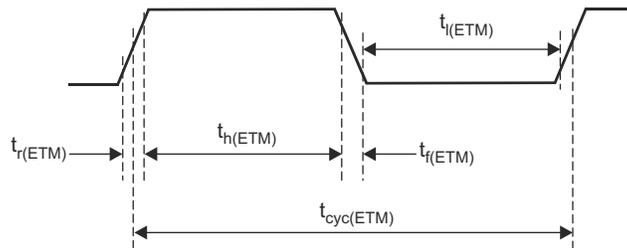
Figure 6-20. ETMTRACECLKOUT Timing
