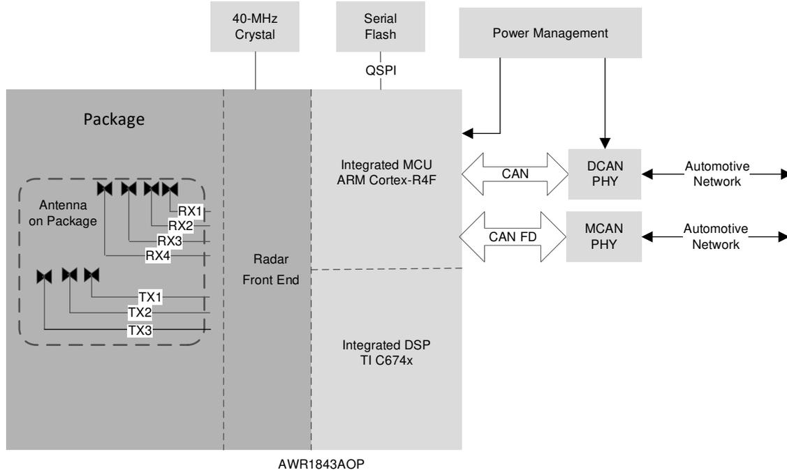
**Figure 2-1. Autonomous Radar Sensor for Automotive Applications**
