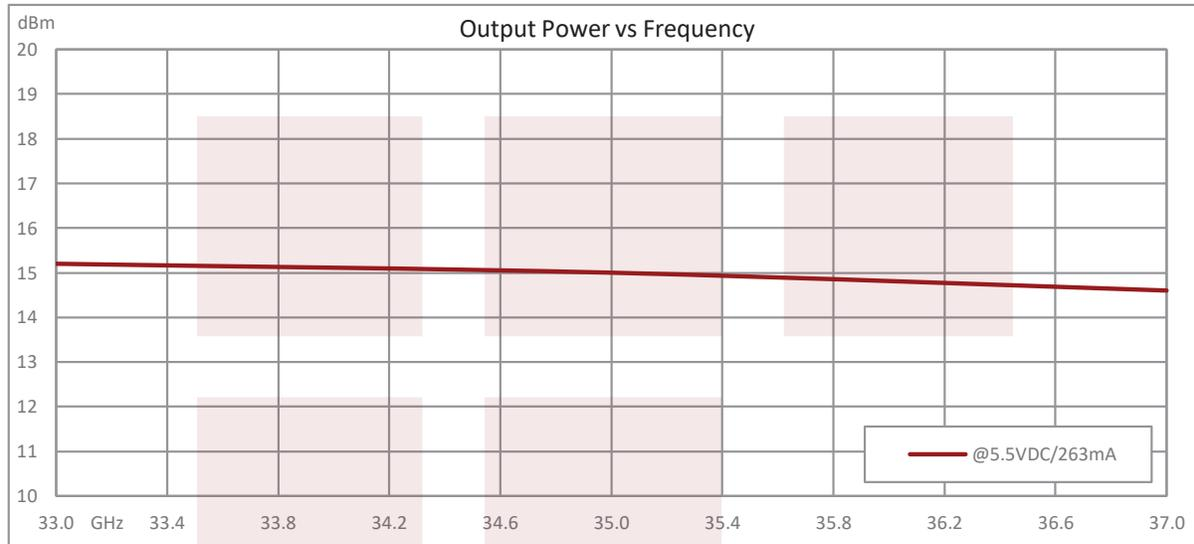
WR-28 Waveguide Gunn Oscillator at a 35 GHz Center Frequency with 3 GHz Tuning Range and -95 dBc/Hz Phase Noise, Ku Band, UG-599/U from Fairview Microwave is in-stock and available to ship same-day. All of our RF/microwave products are available off-the-shelf from our ISO 9001:2008 certified facilities in Lewisville, Texas. Fairview Microwave is RF on-demand.
