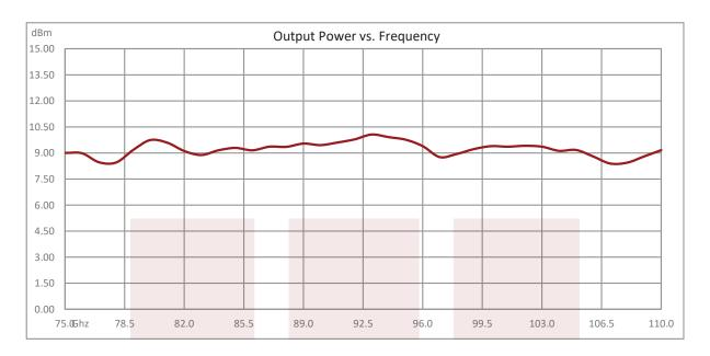
75 GHz to 110 GHz W-Band 6x Active Frequency Multiplier, +10 dBm Pout, WR-19 Output with UG-387/U-M Flange, SMA Female Input from Fairview Microwave is in-stock and available to ship same-day. All of our RF/microwave products are available off-the-shelf from our ISO 9001:2008 certified facilities in Lewisville, Texas. Fairview Microwave is RF on-demand.
