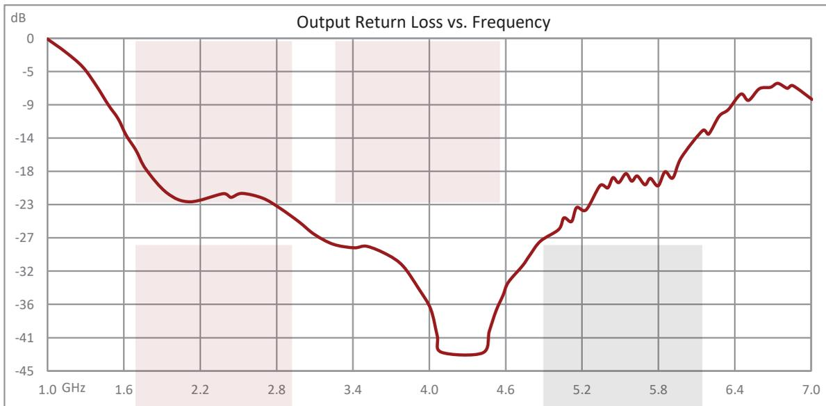
Negative Slope Equalizer, 2 GHz to 6 GHz, 6 dB Fixed Equalizing Value, 0.8 dB Loss, Max Pin 250 mW, SMA from Paster-nack Enterprises has same day shipment for domestic and International orders Our RF, microwave and millimeter wave products maintain a 99.4% availability and are part of the broadest selection in the industry.
