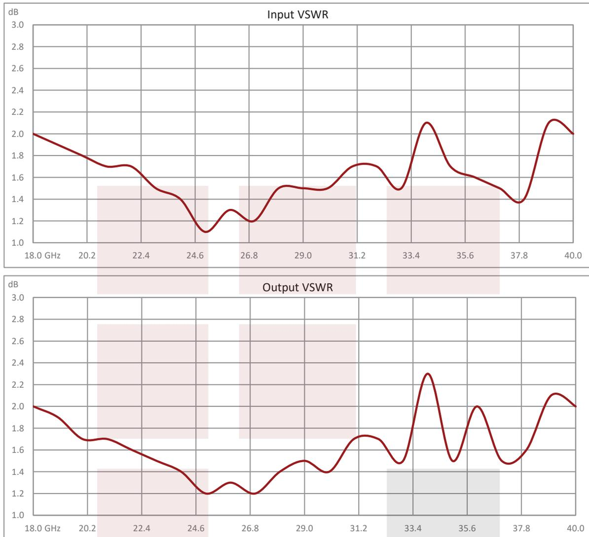
18 GHz to 40 GHz Field Replaceable 2.92mm Positive Slope Equalizer, Max Pin +30, 2 dB Loss and 4 Fixed Equalizing Value from Pasternack Enterprises has same day shipment for domestic and International orders Our RF, microwave and millimeter wave products maintain a 99.4% availability and are part of the broadest selection in the industry.
