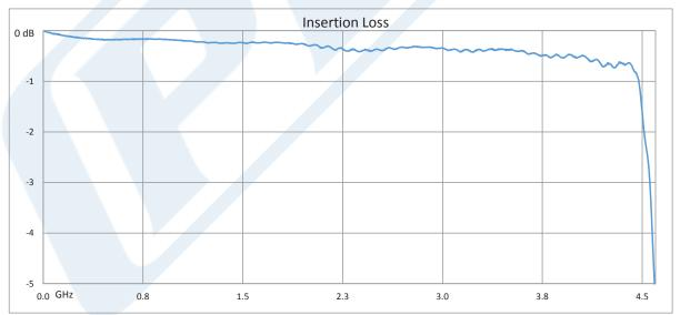
Click the following link (or enter part number in "SEARCH" on website) to obtain additional part information including price, inventory and certifications: 13 Section Lowpass Filter With SMA Female Connectors Operating From DC to 4.4 GHz PE87FL1014
