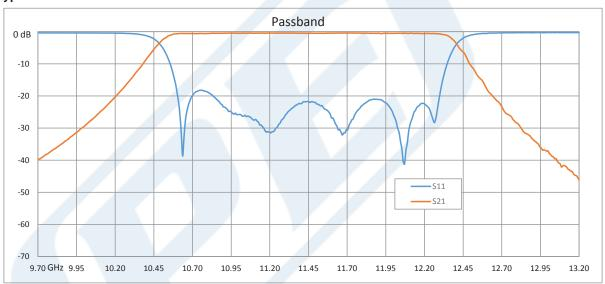
Click the following link (or enter part number in "SEARCH" on website) to obtain additional part information including price, inventory and certifications: 6 Section Bandpass Filter With SMA Female Connectors Operating From 10.7 GHz to 12.2 GHz With a 1.5 GHz Passband PE87FL1003
