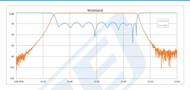
11 Section Bandpass Filter With SMA Female Connectors Operating From 10.55 GHz to 11.8 GHz With a 1.25 GHz Passband from Pasternack Enterprises has same day shipment for domestic and International orders. Our RF, microwave and millimeter wave products maintain a 99% availability and are part of the broadest selection in the industry.
