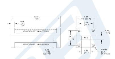
Bandpass Waveguide Filter With WR-42 Interface And a Pass Band From 24.25 GHz to 24.45 GHz from Pasternack Enterprises has same day shipment for domestic and International orders. Our RF, microwave and millimeter wave products maintain a 99% availability and are part of the broadest selection in the industry.
