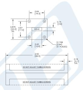
Bandpass Waveguide Filter With WR-42 Interface And a Pass Band From 20.2 GHz to 21.2 GHz from Pasternack Enterprises has same day shipment for domestic and International orders. Our RF, microwave and millimeter wave products maintain a 99% availability and are part of the broadest selection in the industry.
