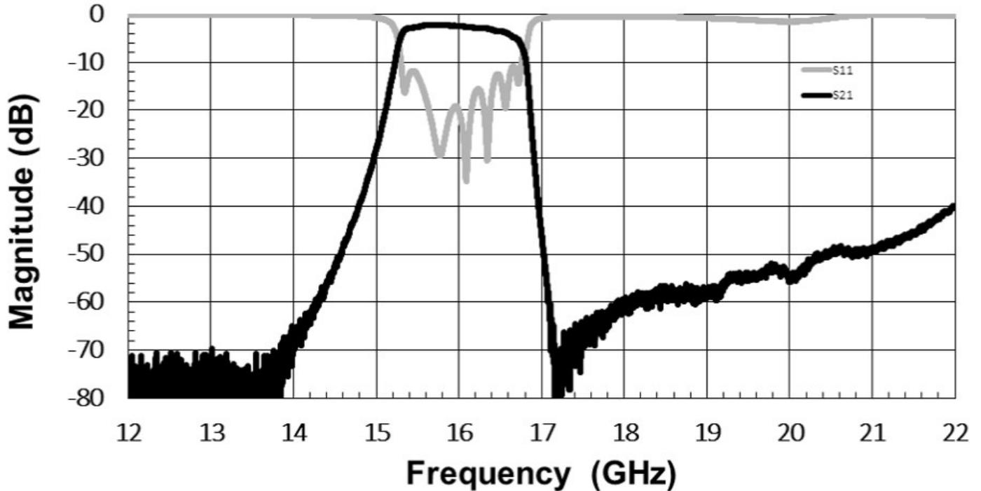
\*Typical de-embedded measured performance mounted on a connectorized test fixture. DEB is 0.010in RO4350B with 50.0Ohm CPW ground traces going into the ports at room temperature.
