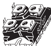
SOT-227[J] Antiparallel Configuration (Isolated Base)
