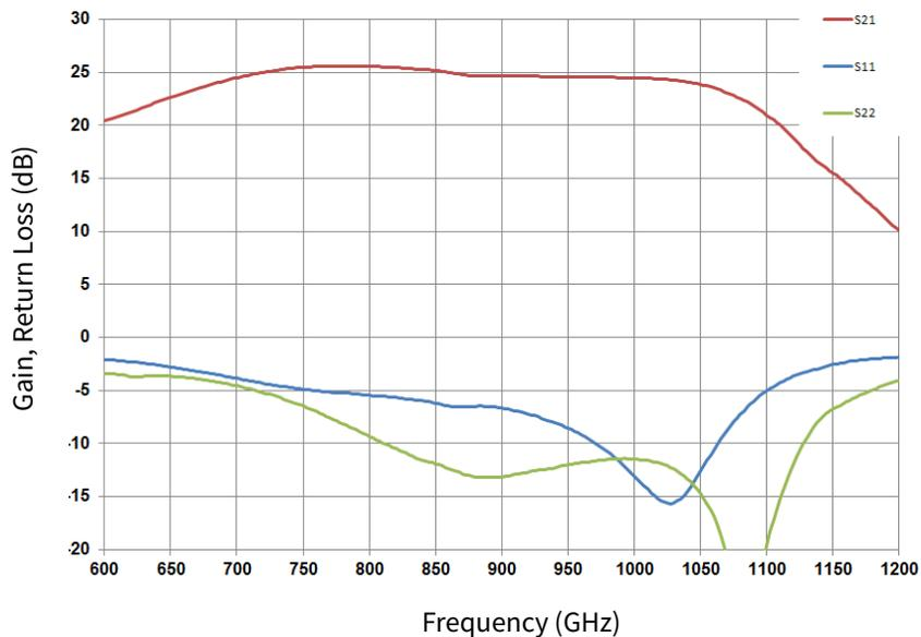
**Figure 1.** Small Signal Gain and Return Loss versus Frequency measured in application circuit CGHV40180F
