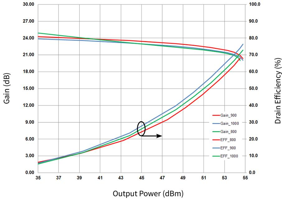
**Figure 3.** Gain and Drain Efficiency vs. Frequency and Output Power
