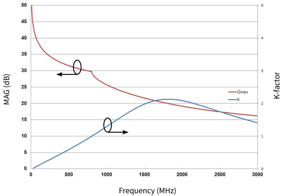
**Figure 4.** Simulated Maximum Available Gain and K-factor of the
