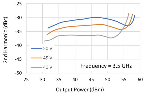
**2<sup>nd</sup> Harmonic vs. Output Power vs. Temperature**
