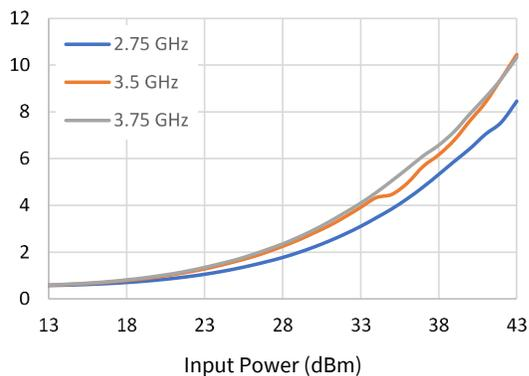
**Gate Current vs. Input Power vs. Frequency**
