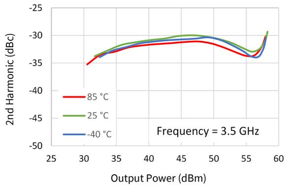
**2<sup>nd</sup> Harmonic vs. Output Power vs.  $V_{DS}$**
