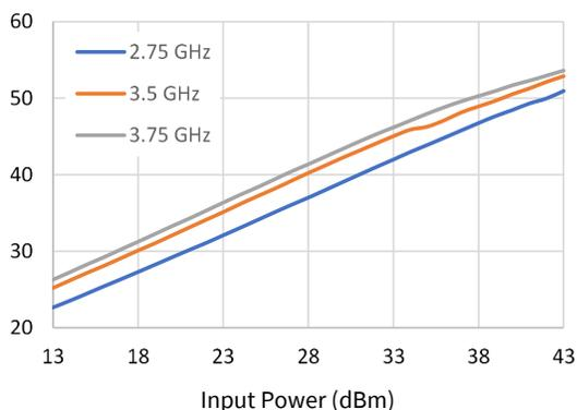
**Drain Efficiency vs. Input Power vs. Frequency**
