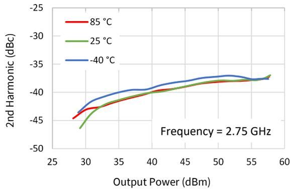
**2<sup>nd</sup> Harmonic vs. Output Power vs.  $V_{DS}$**
