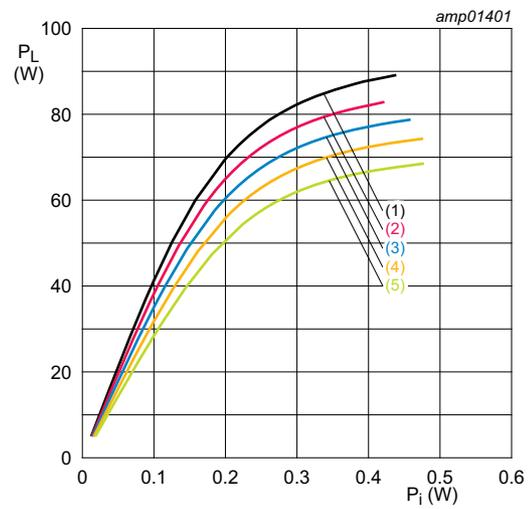
$V_{DS} = 15\text{ V}; I_{Dq} = 893\text{ mA.}$
