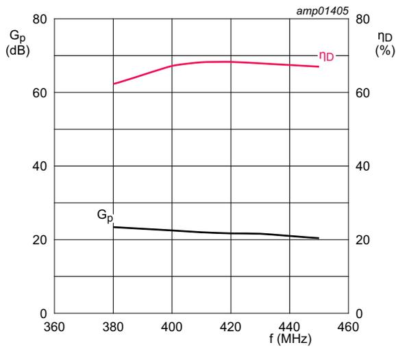
$V_{DS} = 13.6 \text{ V}; I_{Dq} = 80 \text{ mA}; P_L = 55 \text{ W}.$
