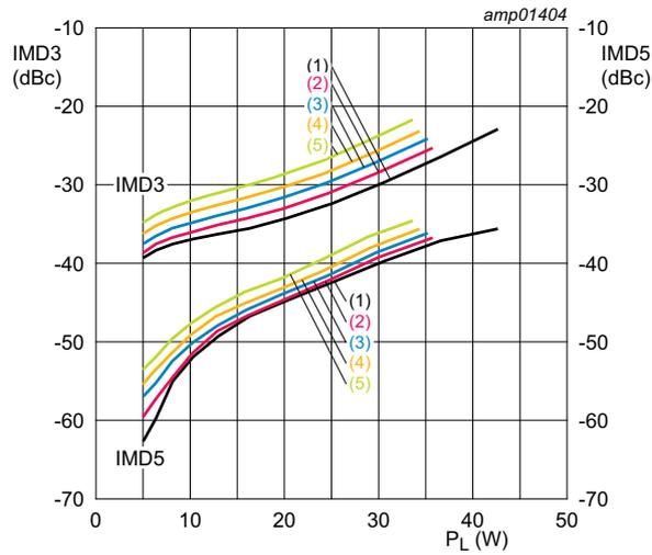
2-Tone signal with 100 kHz carrier separation:  $V_{DS} = 15\text{ V}$ ;  $I_{Dq} = 893\text{ mA}$ .
