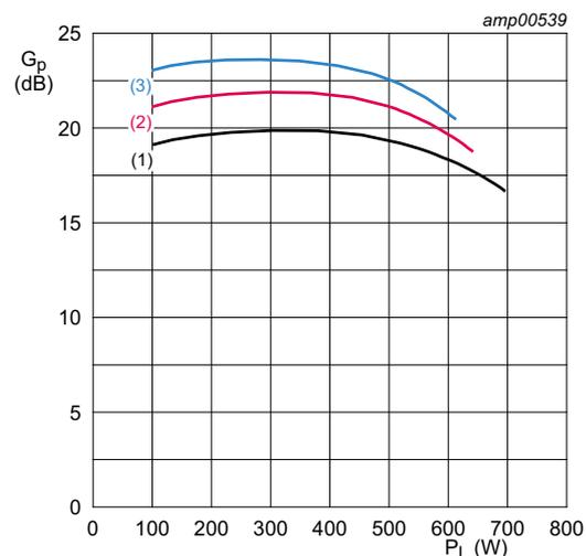
$V_{DS} = 32 \text{ V}$ ;  $I_{Dq} = 400 \text{ mA}$ ;  $t_p = 300 \text{ }\mu\text{s}$ ;  $\delta = 10 \%$ .
