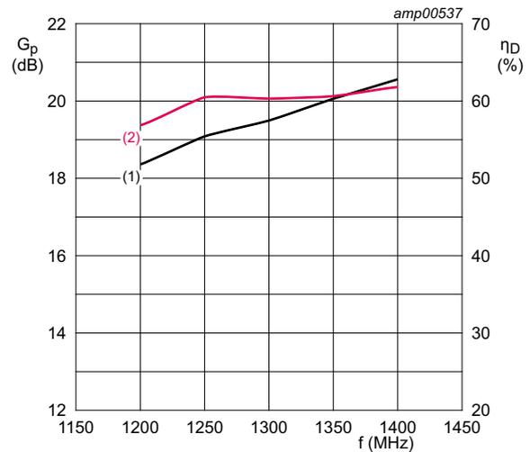
$V_{DS} = 32 \text{ V}$ ;  $I_{Dq} = 400 \text{ mA}$ ;  $t_p = 300 \text{ }\mu\text{s}$ ;  $\delta = 10 \%$ ;  $P_L = 600 \text{ W}$ .
