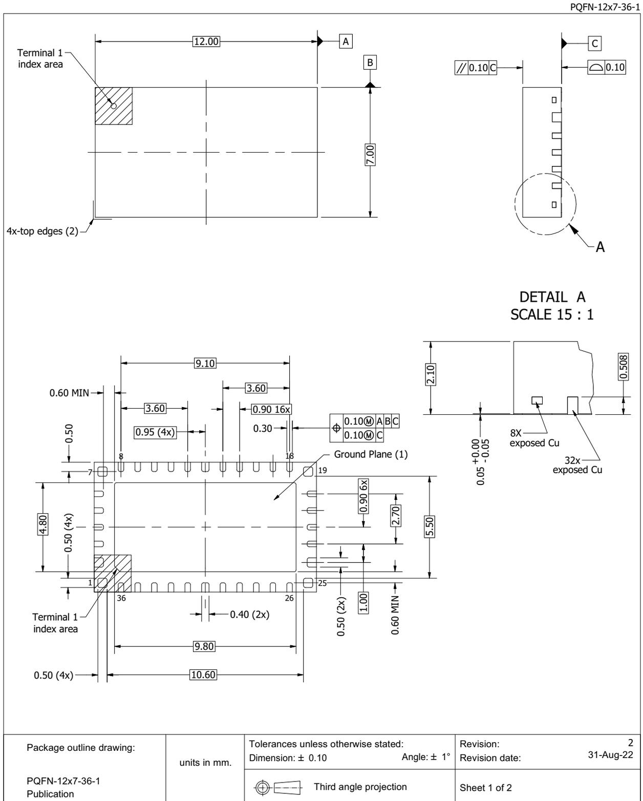
Fig 5. Package outline PQFN-12x7-36-1 (sheet 1 of 2)
