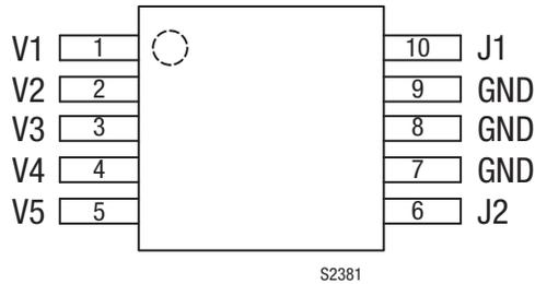
**Figure 2. SKY12322-86LF Pinout (Top View)**
