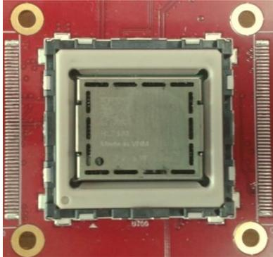
Figure 15. Module in Correct Orientation
