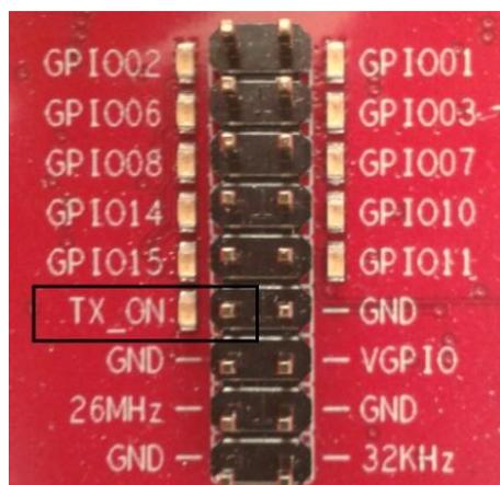
Figure 44. TX-ON Signal
