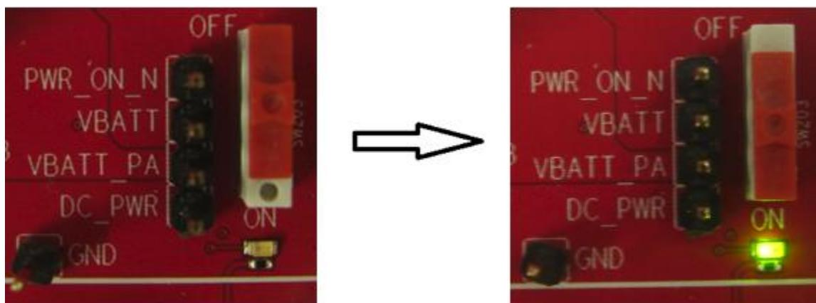
Figure 20. POWER\_ON\_N Pushbutton
