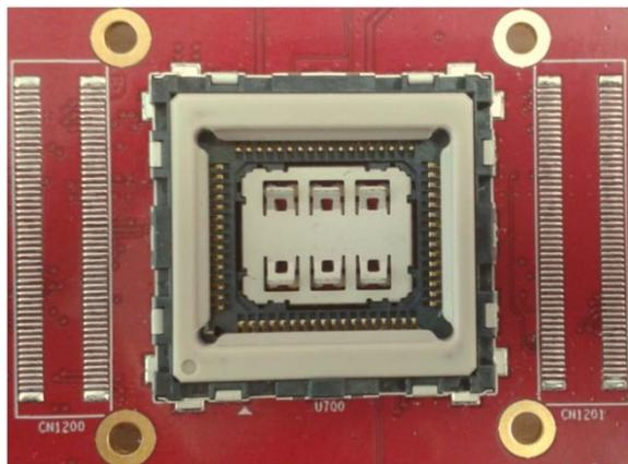
Figure 6. Snap-In Connector with Interposer
