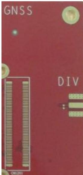
Figure 48. RF Diversity Antenna Connector
