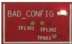
Figure 18. FLASH\_LED for Module in Incorrect Orientation or No Module Present
