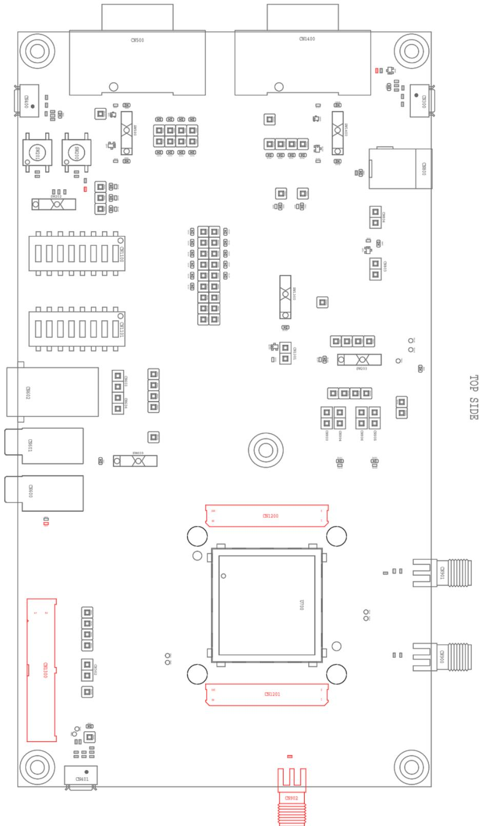
Figure 3. Available Connectors and Components – Top
