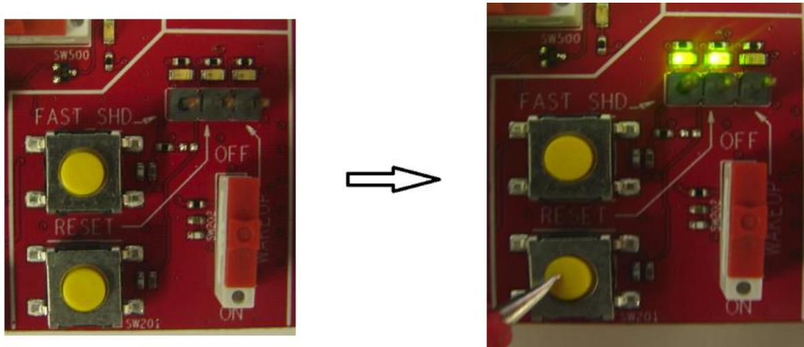
Figure 23. RESET\_IN\_N Pushbutton
