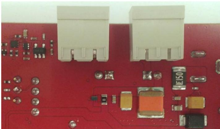
Figure 10. VBATT\_BB and VBATT\_RF Connectors (on the bottom side of the Development Kit)
