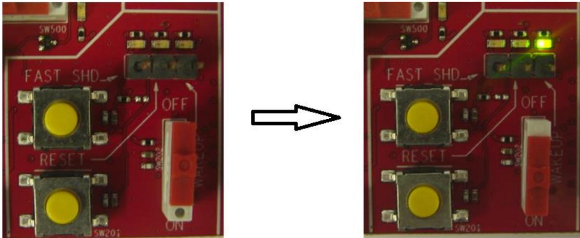
Figure 22. WAKE-UP Pushbutton
