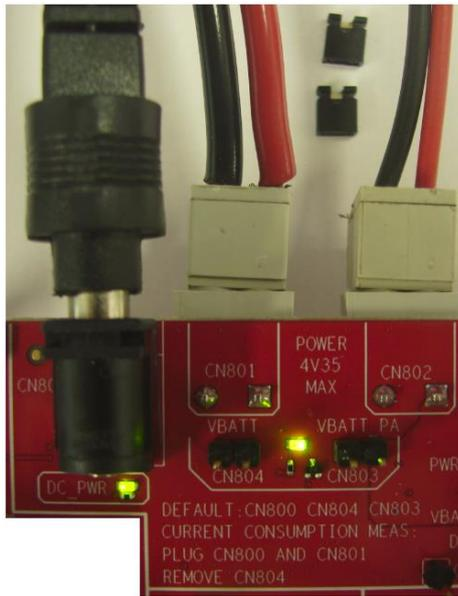
Figure 14. Separate VBATT\_APPLI, VBATT\_BB and VBATT\_RF Configuration
