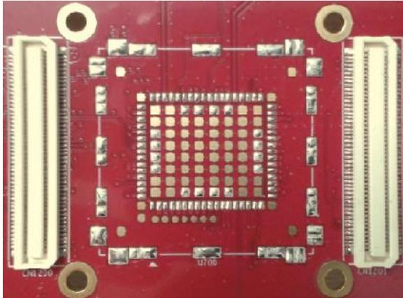
Figure 50. Board To Board Connectors
