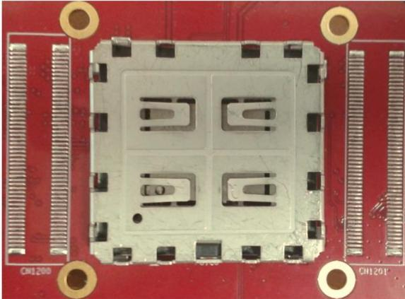
Figure 8. Snap-In Connector with HL78xx Module and Cover
