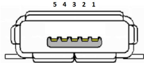
Figure 24. Micro-AB USB Connector
