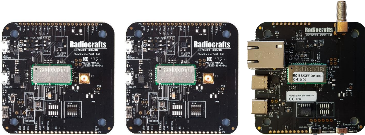
Figure 3. 2 Sensor boards and border router board(right)
