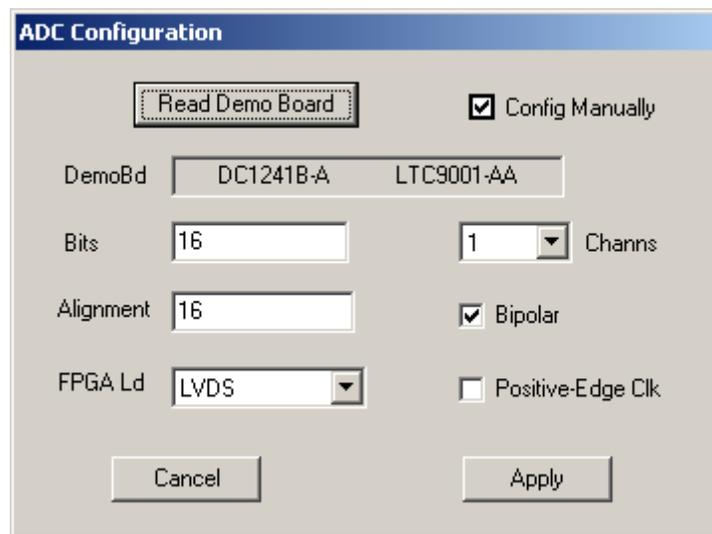
**Figure 2. Entering the correct device information for your ADC. Select the correct parameters for the DC1241. Under normal conditions, PSCOPE should automatically recognize the board and adjust the software settings accordingly.**
