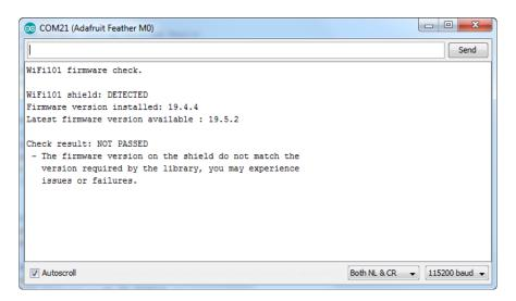
No problem - you can update the firmware through your Arduino/compatible! You must use a 1.8.x version of Arduino IDE. See the orange box below. Start by loading up the FirmwareUpdater sketch
