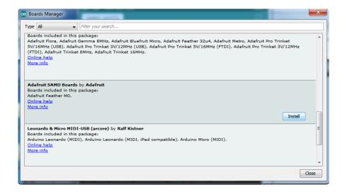
Quit and reopen the Arduino IDE to ensure that all of the boards are properly installed. You should now be able to select and upload to the new boards listed in the Tools->Board menu.
