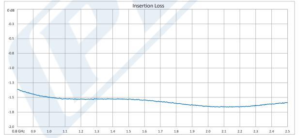
Click the following link (or enter part number in "SEARCH" on website) to obtain additional part information including price, inventory and certifications: Directional 6 dB SMA Coupler From 800 MHz to 2.5 GHz Rated to 50 Watts PE2CP1024-6
