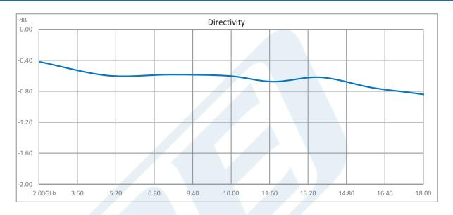
Directional 10 dB SMA Coupler From 2 GHz to 18 GHz Rated to 25 Watts from Pasternack Enterprises has same day shipment for domestic and International orders. Our RF, microwave and millimeter wave products maintain a 99% availability and are part of the broadest selection in the industry.
