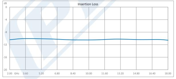
Click the following link (or enter part number in "SEARCH" on website) to obtain additional part information including price, inventory and certifications: Directional 10 dB SMA Coupler From 2 GHz to 18 GHz Rated to 25 Watts PE2215-10
