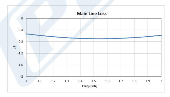
Click the following link (or enter part number in "SEARCH" on website) to obtain additional part information including price, inventory and certifications: Directional 10 dB SMA Coupler From 1 GHz to 2 GHz Rated to 50 Watts PE2201-10
