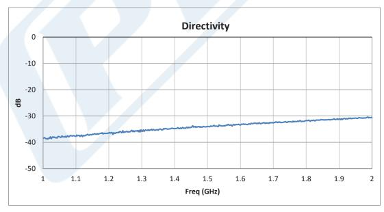
Click the following link (or enter part number in "SEARCH" on website) to obtain additional part information including price, inventory and certifications: Directional 10 dB SMA Coupler From 1 GHz to 2 GHz Rated to 50 Watts PE2201-10
