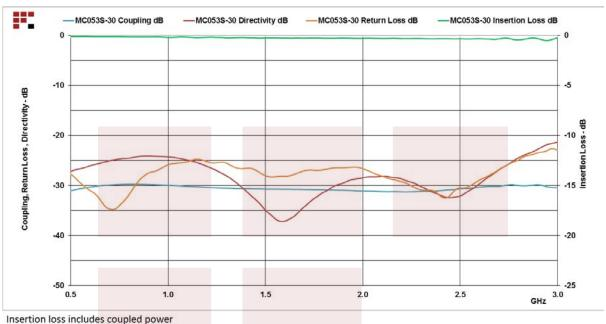
SMA Directional Coupler 30 dB Coupled Port From 500 MHz to 3 GHz Rated To 50 Watts from Fairview Microwave is instock and available to ship same-day. All of our RF/microwave products are available off-the-shelf from our ISO 9001: 2008 certified facilities in Allen, Texas. Fairview Microwave is RF on-demand.
