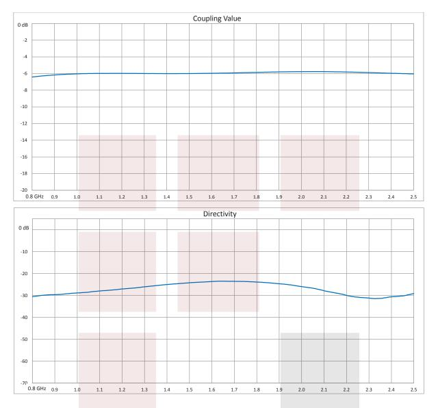
SMA Directional Coupler 6 dB Coupled Port From 800 MHz to 2.5 GHz Rated To 50 Watts from Fairview Microwave is instock and available to ship same-day. All of our RF/microwave products are available off-the-shelf from our ISO 9001:2008 certified facilities in Allen, Texas. Fairview Microwave is RF on-demand.
