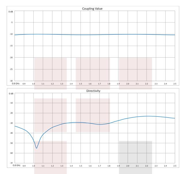
N Directional Coupler 10 dB Coupled Port From 800 MHz to 2.5 GHz Rated To 60 Watts from Fairview Microwave is in-stock and available to ship same-day. All of our RF/microwave products are available off-the-shelf from our ISO 9001:2008 certified facilities in Allen, Texas. Fairview Microwave is RF on-demand.
