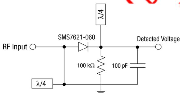
Figure 2. Schematic of a 24 GHz Detector Design
