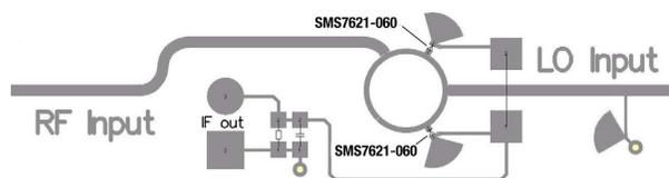
Figure 5. Layout for a 24 GHz Rat-Race Mixer
