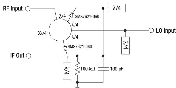
Figure 4. Schematic of a 24 GHz Rat-Race Mixer
