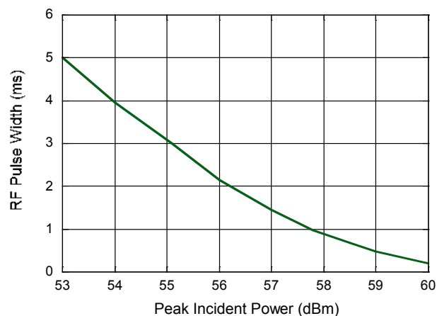
Pulse Width vs. Peak Input Power @ +85°C (10% Duty Cycle, 1.3 GHz)
