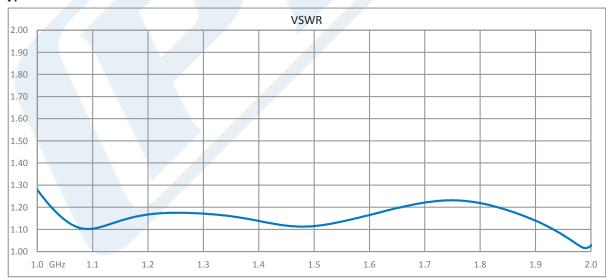
Click the following link (or enter part number in "SEARCH" on website) to obtain additional part information including price, inventory and certifications: Circulator with 18 dB Isolation from 1 GHz to 2 GHz, 10 Watts and SMA Female PE8400
