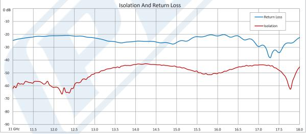
Click the following link (or enter part number in "SEARCH" on website) to obtain additional part information including price, inventory and certifications: Dual Junction Isolator With 40 dB Isolation From 11 GHz to 18 GHz, 5 Watts And SMA Female PE83IR1024
