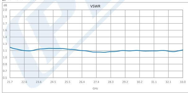
Click the following link (or enter part number in "SEARCH" on website) to obtain additional part information including price, inventory and certifications: WR-34 Waveguide Circulator, 21.7 GHz to 33 GHz, 18 dB min Isolation, Cover Flange, Aluminum PE-W34CR001
