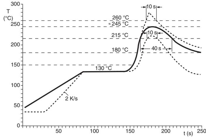
Fig. 8 - Soldering Reflow with Sn Solder
