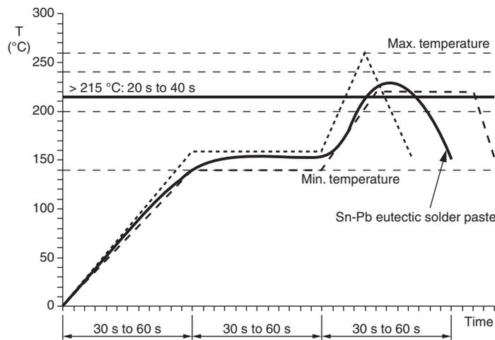
Fig. 7 - Soldering IR Reflow with SnPb Solder
