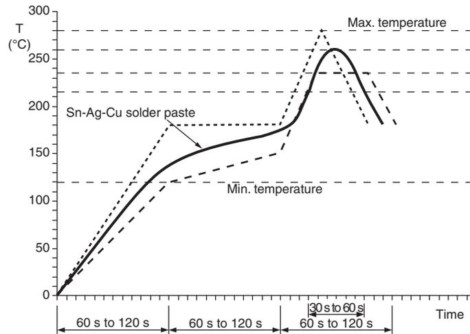
Fig. 9 - Soldering IR Reflow with SnAgCu Solder
