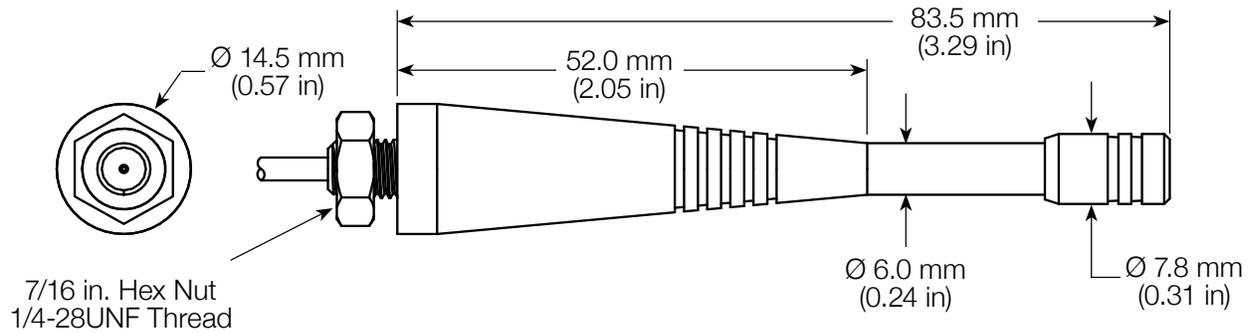
Figure 6: PW LTE Band 5 Antenna Dimensions
