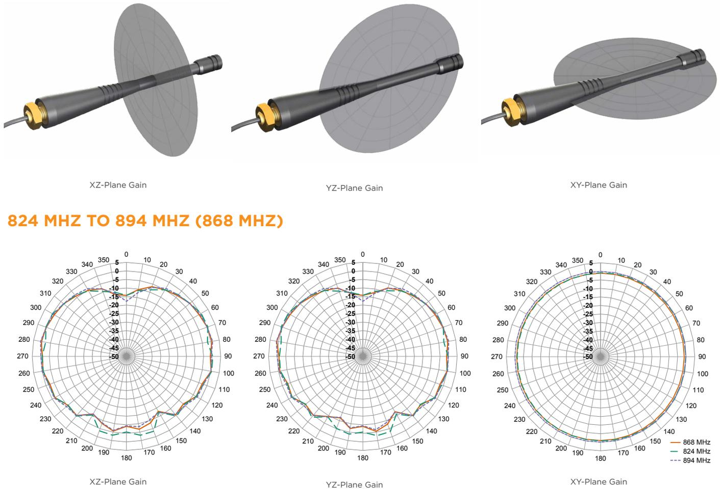
Figure 8: Radiation Patterns for PW LTE Band 5 Antenna
