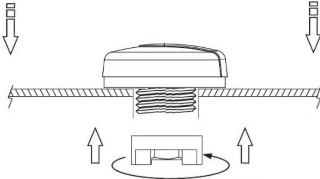
Recommended torque for Mounting is 3.92N·m
