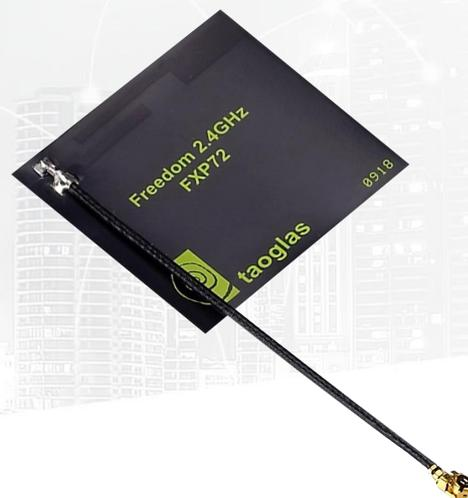
The FXP72 Freedom 2.4GHz Antenna works on Wi-Fi, ZigBee, Bluetooth and ISM band at 2.4GHz. This antenna has been designed as a general solution to cover the current market applications, with easy installation through a cable connection. The antenna has been designed to work on different plastics material and thickness. We have selected a piece of ABS plastic with 2mm of thickness as a baseline for testing.
