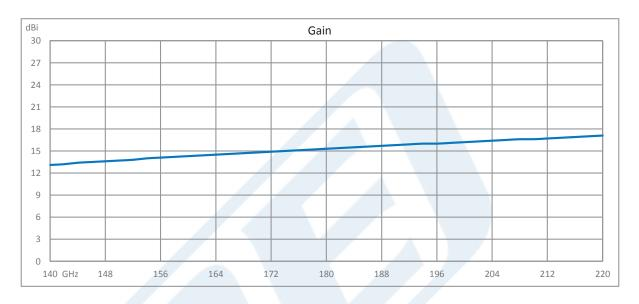
WR-5 Waveguide Conical Gain Horn Antenna Operating from 140 GHz to 220 GHz with a Nominal 15 dBi Gain with UG-387/U Round Cover Flange from Pasternack Enterprises has same day shipment for domestic and International orders. Our RF, microwave and millimeter wave products maintain a 99.4% availability and are part of the broadest selection in the industry.
