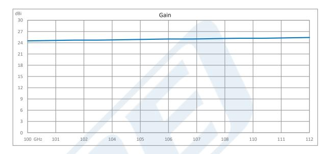
WR-8 Waveguide Conical Gain Horn Antenna Operating from 100 GHz to 112 GHz with a Nominal 25 dBi Gain with UG-387/U-Mod Round Cover Flange from Pasternack Enterprises has same day shipment for domestic and International orders. Our RF, microwave and millimeter wave products maintain a 99.4% availability and are part of the broadest selection in the industry.
