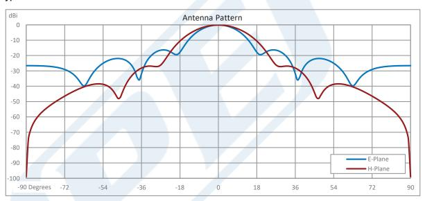
Click the following link (or enter part number in "SEARCH" on website) to obtain additional part information including price, inventory and certifications: WR-10 Waveguide Conical Gain Horn Antenna Operating from 77 GHz to 87 GHz with a Nominal 20 dBi Gain with UG-387/U Round Cover Flange PEWAN1055
