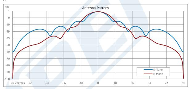
Click the following link (or enter part number in "SEARCH" on website) to obtain additional part information including price, inventory and certifications: WR-12 Waveguide Conical Gain Horn Antenna Operating from 77 GHz to 87 GHz with a Nominal 20 dBi Gain with UG-387/U Round Cover Flange PEWAN1047
