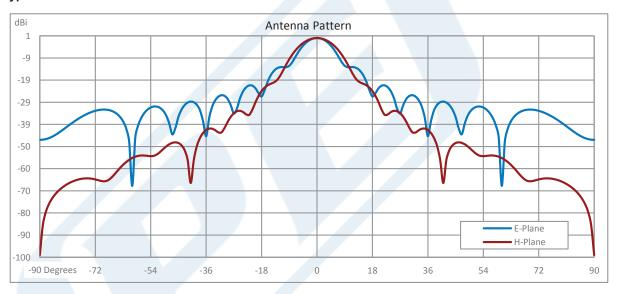
Click the following link (or enter part number in "SEARCH" on website) to obtain additional part information including price, inventory and certifications: WR-19 Waveguide Conical Gain Horn Antenna Operating from 50 GHz to 58 GHz with a Nominal 25 dBi Gain with UG-383/U-Mod Round Cover Flange PEWAN1036
