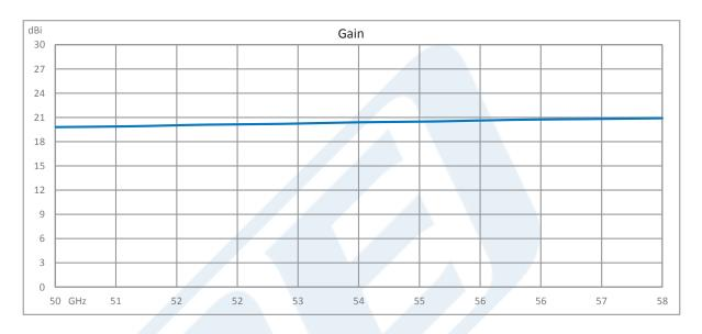
WR-19 Waveguide Conical Gain Horn Antenna Operating from 50 GHz to 58 GHz with a Nominal 20 dBi Gain with UG-383/U-Mod Round Cover Flange from Pasternack Enterprises has same day shipment for domestic and International orders. Our RF, microwave and millimeter wave products maintain a 99.4% availability and are part of the broadest selection in the industry.
