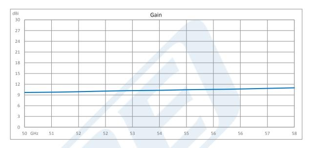
WR-19 Waveguide Conical Gain Horn Antenna Operating from 50 GHz to 58 GHz with a Nominal 10 dBi Gain with UG-383/U-Mod Round Cover Flange from Pasternack Enterprises has same day shipment for domestic and International orders. Our RF, microwave and millimeter wave products maintain a 99.4% availability and are part of the broadest selection in the industry.
