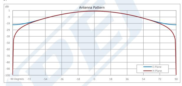
Click the following link (or enter part number in "SEARCH" on website) to obtain additional part information including price, inventory and certifications: WR-19 Waveguide Conical Gain Horn Antenna Operating from 50 GHz to 58 GHz with a Nominal 10 dBi Gain with UG-383/U-Mod Round Cover Flange PEWAN1033
