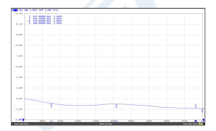
Click the following link (or enter part number in "SEARCH" on website) to obtain additional part information including price, inventory and certifications: 2.15 dBi, UHF Rubber Duck Antenna, 412-480 MHz, SMA Female Connector, Vertical Polarization PEANRBD1011
